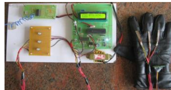
Transmitter block of gloves based dumb assist device
